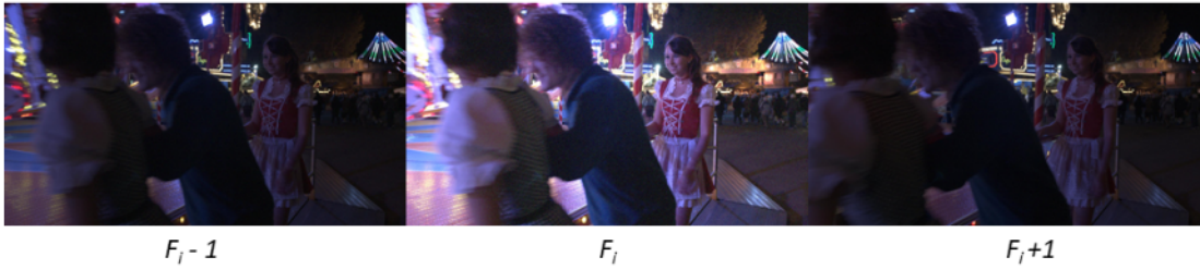
Figure 3.3: Representation of three consecutive frames with two alternate exposures of the carousel firework scene in Froehlich et al. (2014) HDR dataset. Each frame in three consecutive frame input contain some missing contents with the Presence of noise in frame F_i - 1 and F_i + 1 in the darker region due to acquisition with low exposure whereas F_i , which was taken with high exposure, lacks details in over-saturated and bright regions. The missing content of a final HDR image has to be reconstructed from neighboring frames with alternating exposures.
