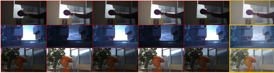
Figure 1.4: Represents conventional camera consecutive frames with alternating exposures highlighted in red. The over-exposed frames have regions where all the information is lost while in case low exposure frames, the information is suppressed in shadow regions of the frames. The goal of the the HDR reconstruction method is to recover the lost details in both under and over-exposed regions from LDR frames.
