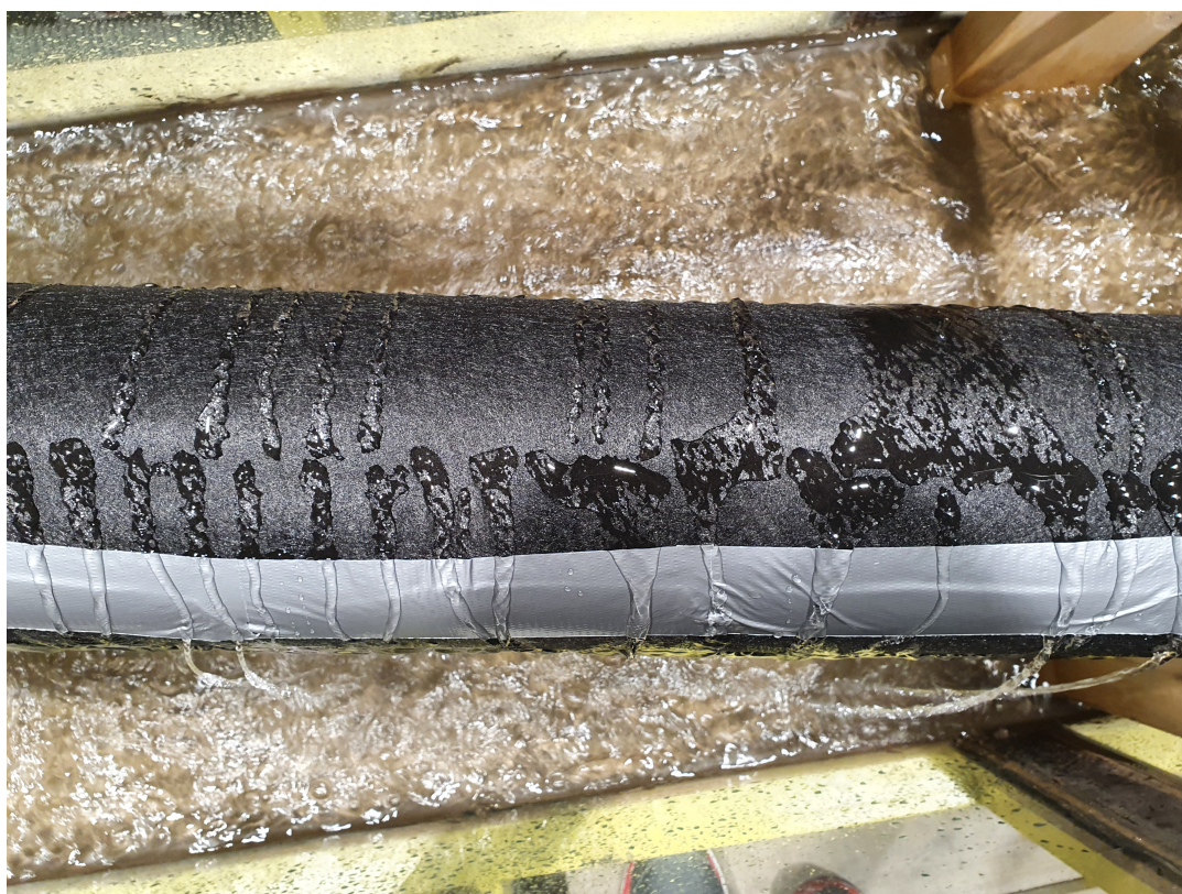
Figure A3.6: A run with the geotextile. Seen from above. Photo credits: Ida Hovland Haveraaen
