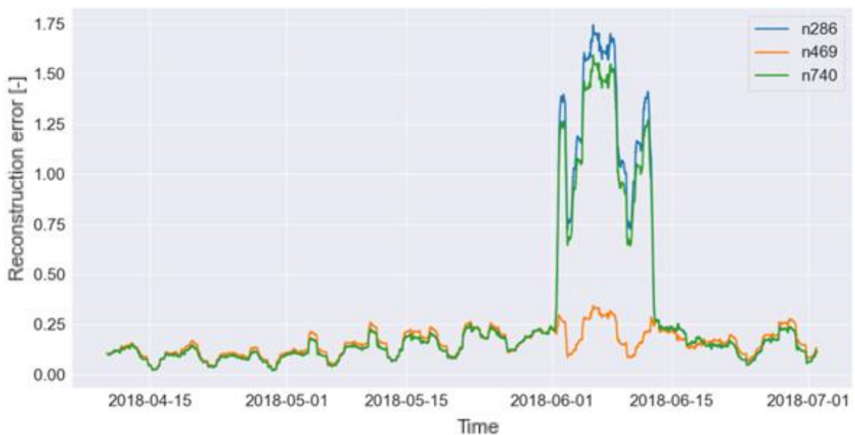
Figure 16 Rolling mean on a per day basis for the reconstruction error from sensors n286, n469, and n740 with the leak in pipe 866.
