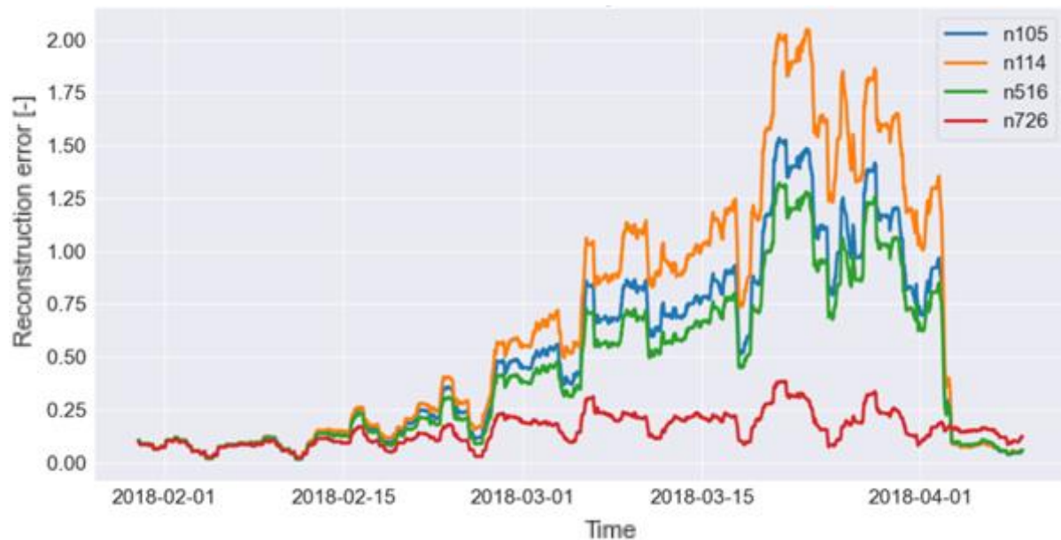
Figure 11 Rolling mean on a per day basis for the reconstruction error from sensors n105, n114, n616 and n726 with the leak in pipe 461.
