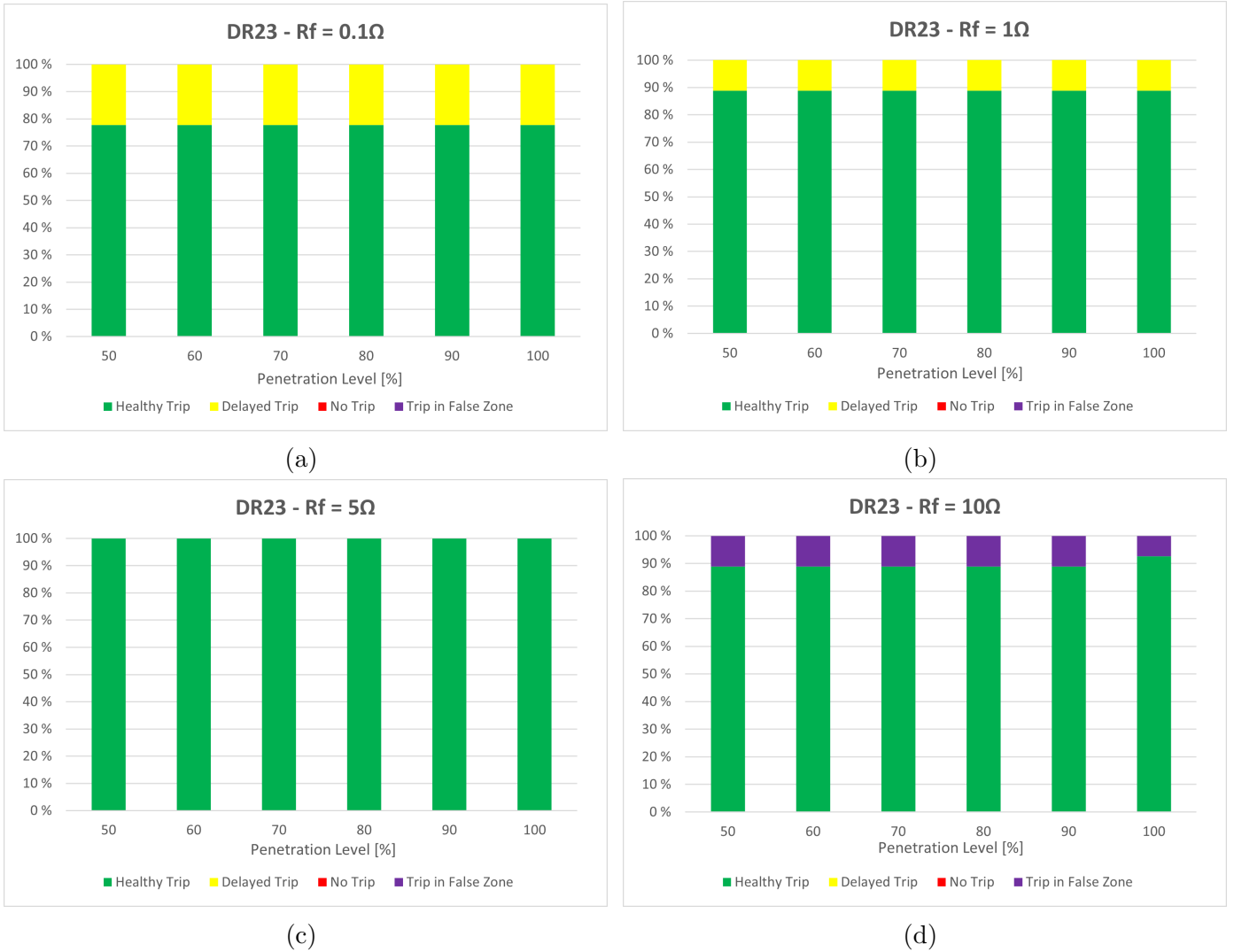
Figure 22: Impact of fault resistance on DR23, including simulations for unsymmetrical faults only, all control strategies, and divided between all penetration levels. a) R_f = 0.1\Omega , b) R_f = 1\Omega , c) R_f = 5\Omega and d) R_f = 10\Omega .
