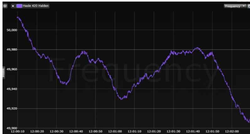
Figure 5.4: Frequency variations during ambient conditions at the interconnection Hasle-Halden on a 2 minute interval measured by PMU.
