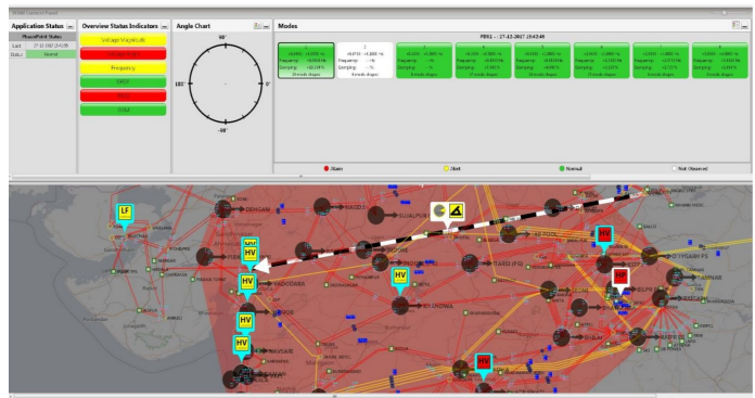
Figure 13: Indian monitoring tool displaying phasors as well as other stability indicators on the GIS [6].
