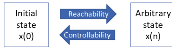
Figure 17: Reachability refers to the ability to go from initial state to an arbitrary state by means of a sequence of control inputs and the controllability matrix. Controllability refers to the ability to go from an arbitrary state to the initial state, and is only possible if A is invertible.
