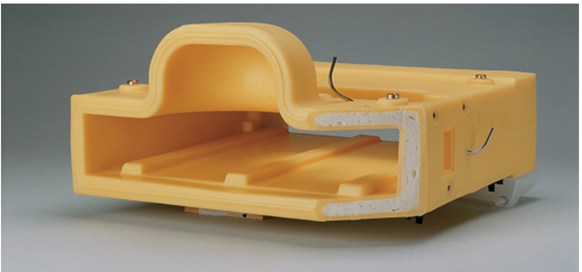
FIGURE 27. ROTATIONAL MOULDED PART WITH FOAM FILLING, 2022, GREGSTROM CORPORATION. HTTP://GREGSTROM.COM/ROTATIONAL-MOLDING/
