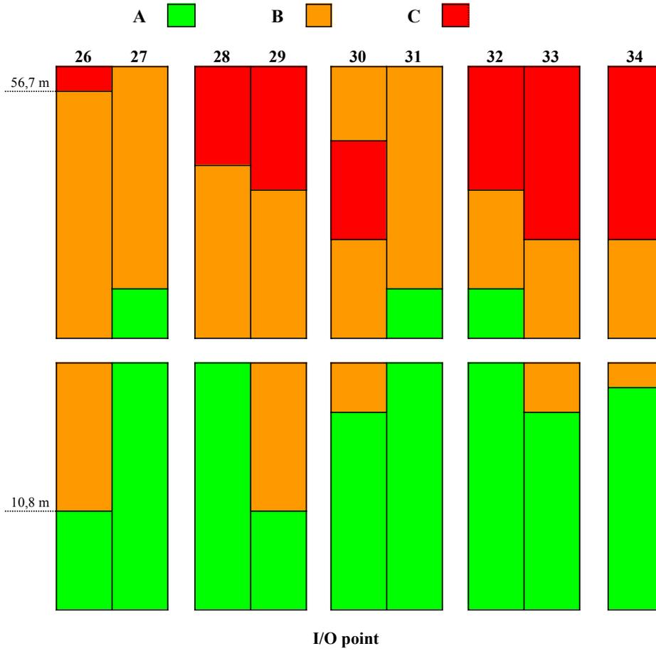
Figure 4.20: The zones A, B and C for the relevant racks for reshuffling in the carton picking area. The figure shows rack 26-34 at the ground level (shelf 1) as seen from above. To the left, the distances from the beginning of zone A to the beginning of zone B and C for rack 26 is shown to illustrate the lengths.
