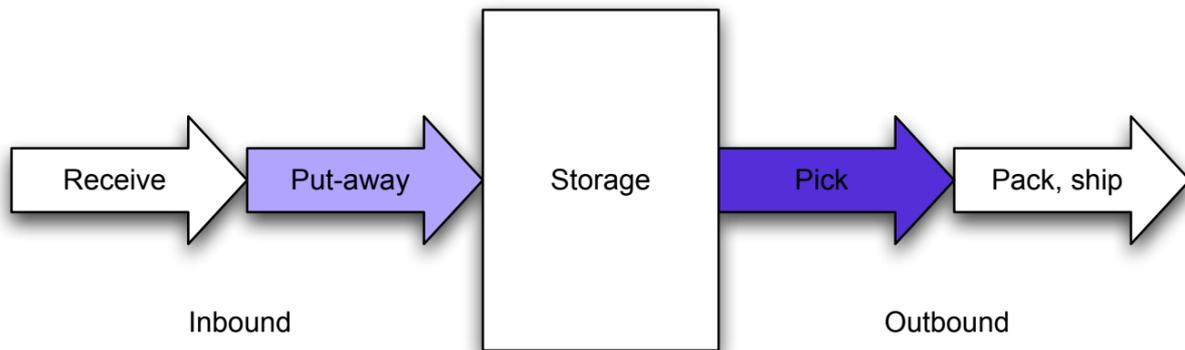
Figure 3.2: A simplified illustration of the warehouse operations, adapted from (Bartholdi and Hackman, 2019, page 24).
