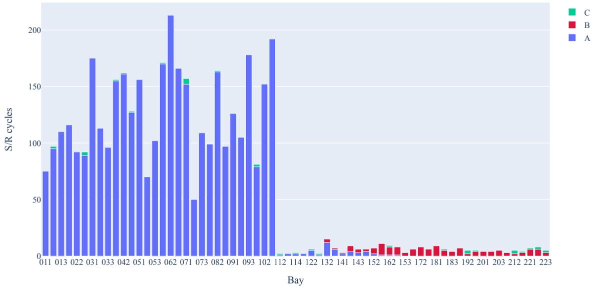
Figure 4.13: The total amount of S/R cycles per bay for rack number 27 in 2021 for the carton picking in each class A, B, and C.
