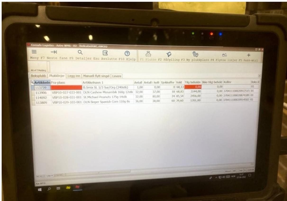
Figure 4.8: An image of the screen attached to the forklifts used by the operators. Here, an order is shown with four picking-lines. The lines contain information about the different products in the order, including storage location, name, amount to pick and amount available, weight, etc.
