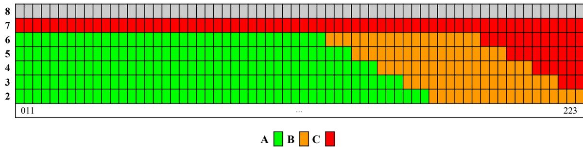
Figure 4.5: An illustration showing the locations of the classes A, B and C on shelves 2 to 8 of the storage area, as seen from the side. The gray areas corresponds to class D.
