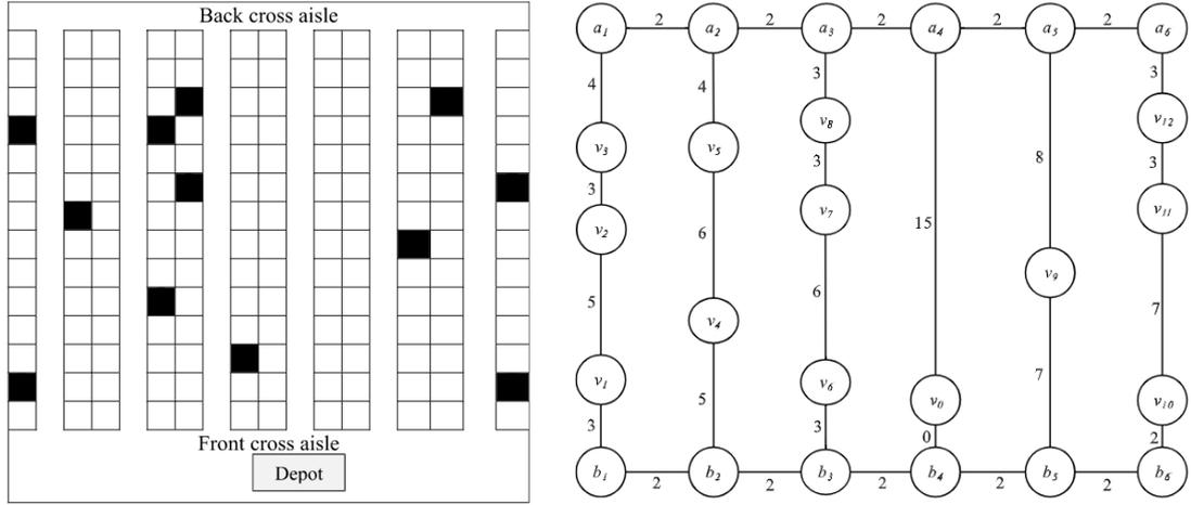
(a) Layout of a conventional warehouse with a single block. The black squares shows the picking locations in an example order. (b) Graph representation  $G$  of the example layout in figure (a), where  $m = 12$  and  $n = 6$ .
