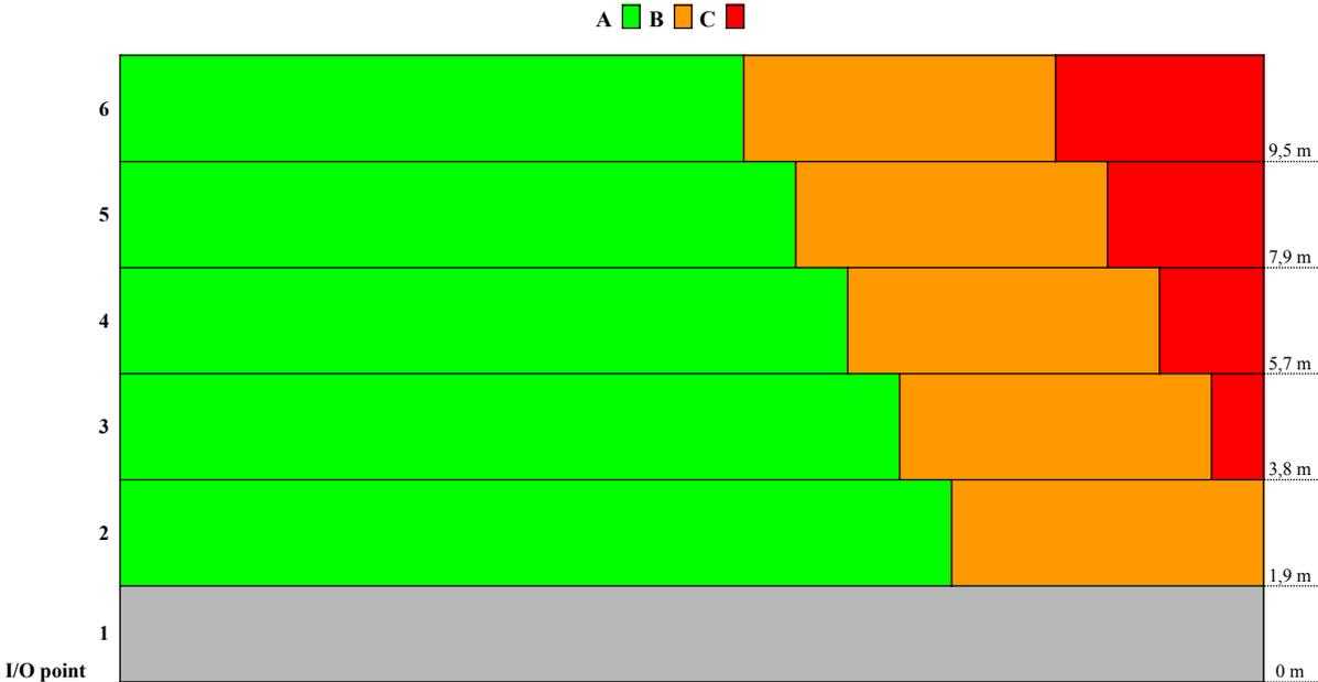
Figure 4.19: The zones A, B and C for the relevant shelves for reshuffling in the full pallet area. The figure shows one arbitrary rack as seen from the side with the corresponding zones (the zones are similar for all relevant racks). The heights in the bottom of each shelf are shown to the right of the figure. Shelf number 1 is shown in grey because it is not relevant for the analyses in this area.
