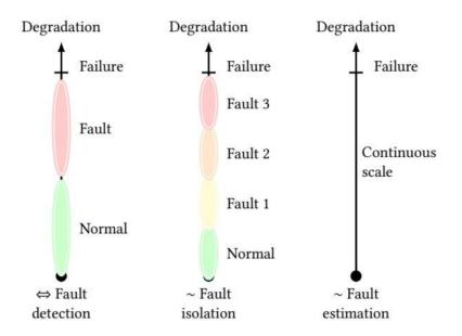
Figure 8: Degradation indicator models.
