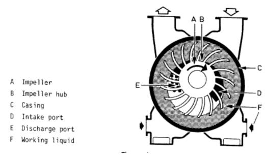
Figure 17: Liquid ring compressor operating mechanism.
