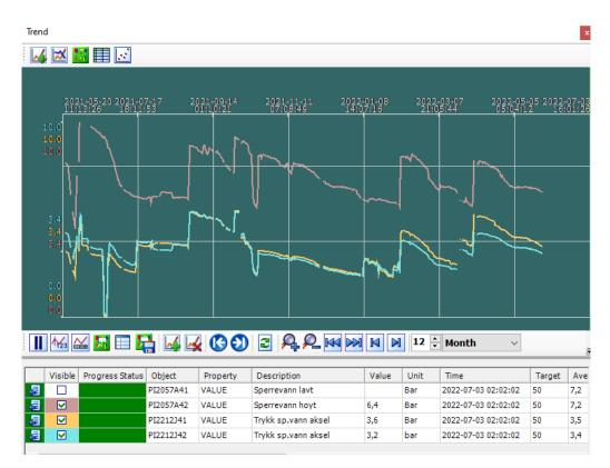
Figure 27: Compressor J: Seal water pressure vs. seal water supply pressure
