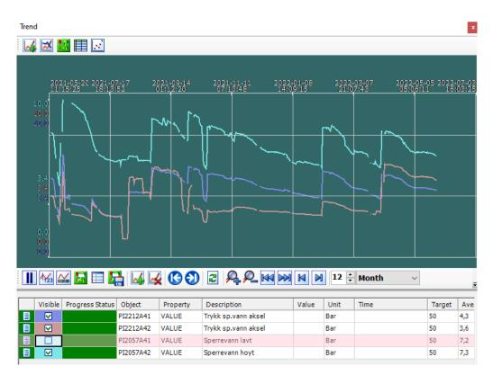
Figure 29: Compressor A: Seal water pressure vs. seal water supply pressure
