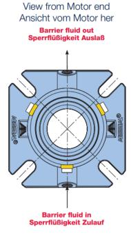
Figure 25: Mechanical seal drawing
