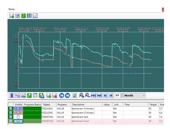
Figure 28: Compressor I: Seal water pressure vs. seal water supply pressure
