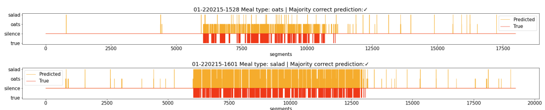
Figure 33: 3C system predicted and true labels for two recordings: oats meal (top), salad meal (bottom). The yellow labels indicate the predictions, which were either class “silence”, “salad” or “oats”. The true labels in red show two classes “silence” or “chew”. For the true labels all of the chews are of the meal type indicated by the title of the recording.
