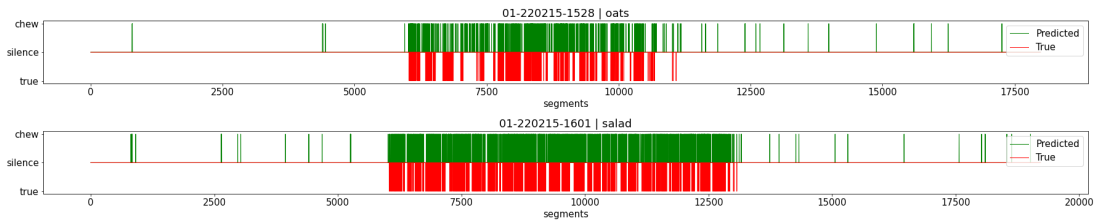
Figure 31: Chew detector predicted and true labels for two testing recordings: oats meal (top), salad meal (bottom). The green labels indicate the predictions, which were either class “silence” or “chew”. The red labels are the true labels, and are provided for reference.
