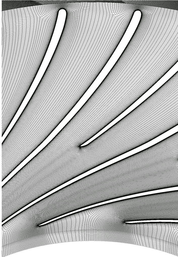
Figure C.5: Runner passage mesh.
