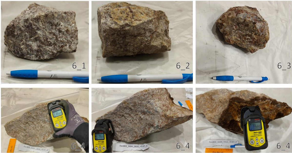
Figure 3-3 Shows the four higher radioactive specimens and three different images of specimen 6_4 to illustrate the slight difference in measured \mu\text{Sv/h} depending on where the detector is placed on the specimen.
