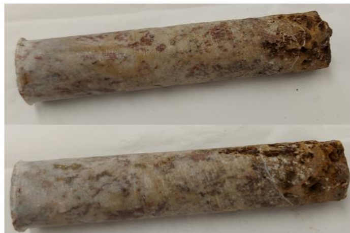
Figure 3-12 Two pictures of the 28 mm wide core made from specimen 6_4 (Figure 3-3) that was used for \mu CT. It was drilled down from the eroded side of the specimen.
