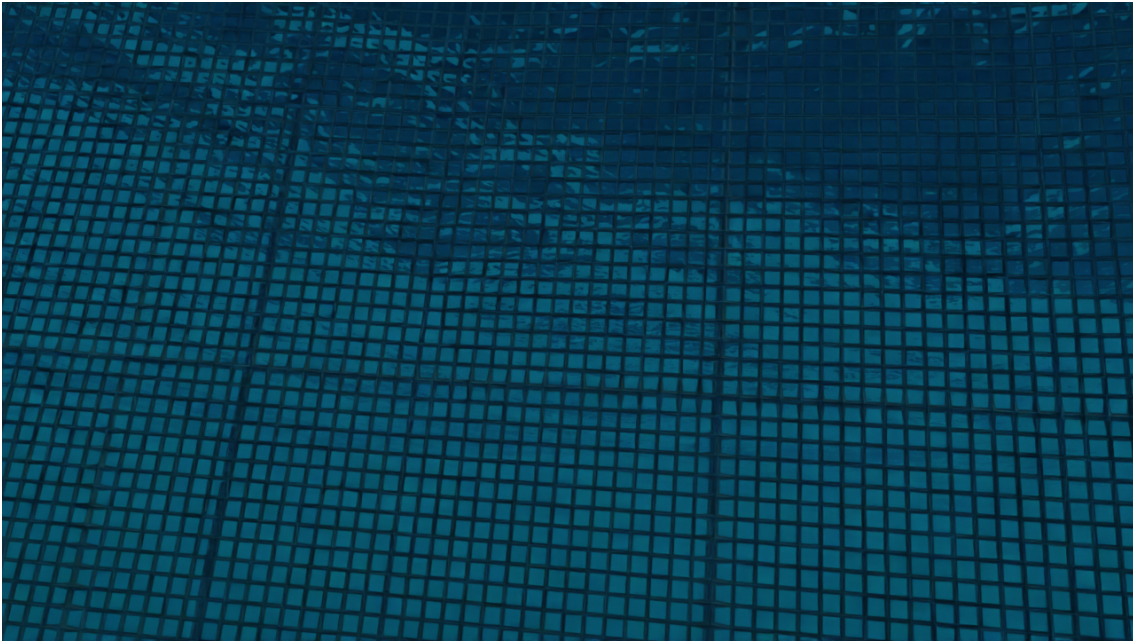
Figure 3.4: Rendering of the net structure. Thicker support ropes are shown both horizontally and vertically. Additionally there are ropes outside the net structure supporting the bottom weight ring.
