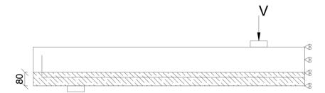
Figure 3.11 – Beam S1D18a108 with tension stiffening zone
