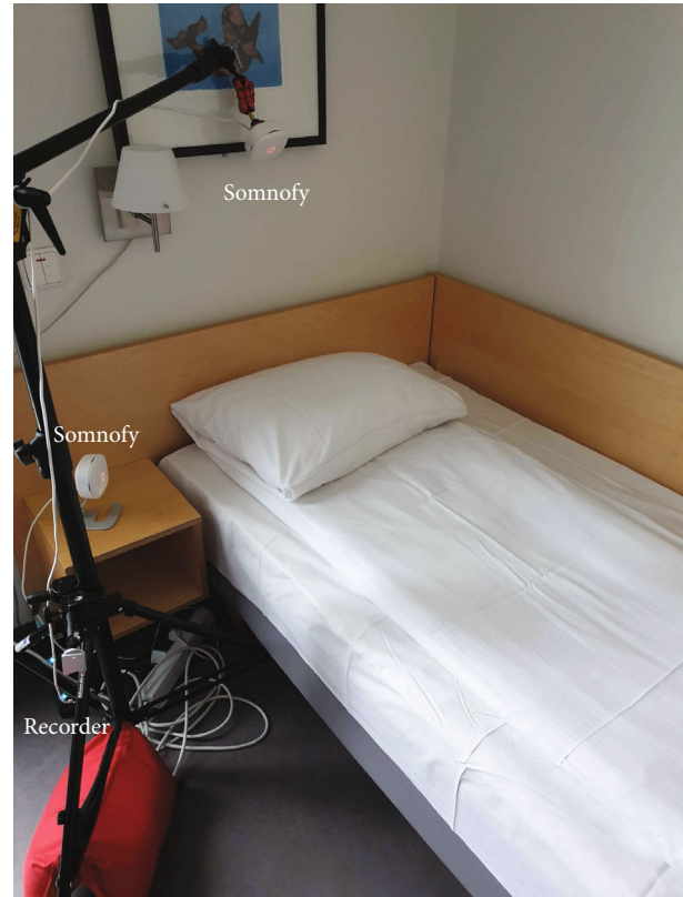
FIGURE 1: A visualization of the Somnofy set up. One Somnofy unit was placed on the nightstand, and one unit mounted in a wall position. Both units were aiming towards the participants' chest from approximately one meter. Both units were connected to a Somnofy Recorder placed under the nightstand.
