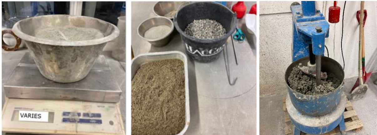
Figure 3-5 The different components were weighed and then mixed. Picture illustrating the mixing process, a mix where it was necessary to add extra water is shown.
