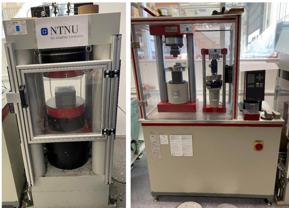
Figure 3-7 To the left a standard compressive strength test machine. To the right the combined compressive and tensile strength test machine.
