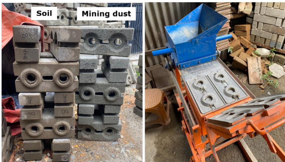
Figure 5-10 Left picture: CSEB with soil and mining dust. Right picture: One type of press. Several different alternatives exist, and they can produce from one to three earth blocks at a time .
