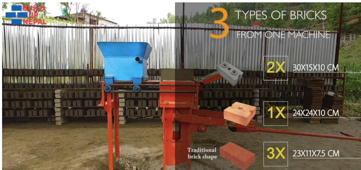
Figure 2-15 Illustration of a machine used to make CSEB, and three different blocks that can be made using the same machine [69].
