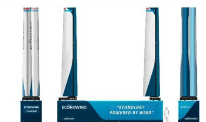
Figure 2.8: Containerized ventifoil unit
