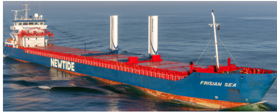
Figure 2.5: Vessel installed with Econowind Ventifoils
