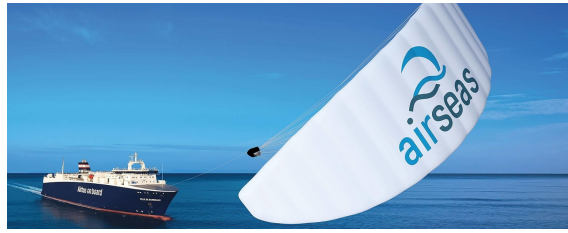
Figure 2.6: Concept for kites in cargo transportation systems
