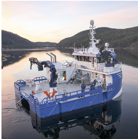
Figure 3: Picture of the Frøy Multi, a typical work or service boat. The wide working deck and the deck equipment can be seen. (Frøy n.d.d)
