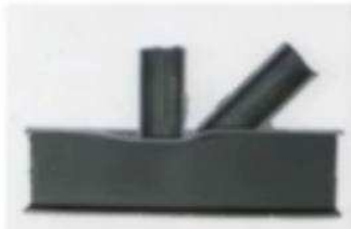
Chord face deformation (yielding)
