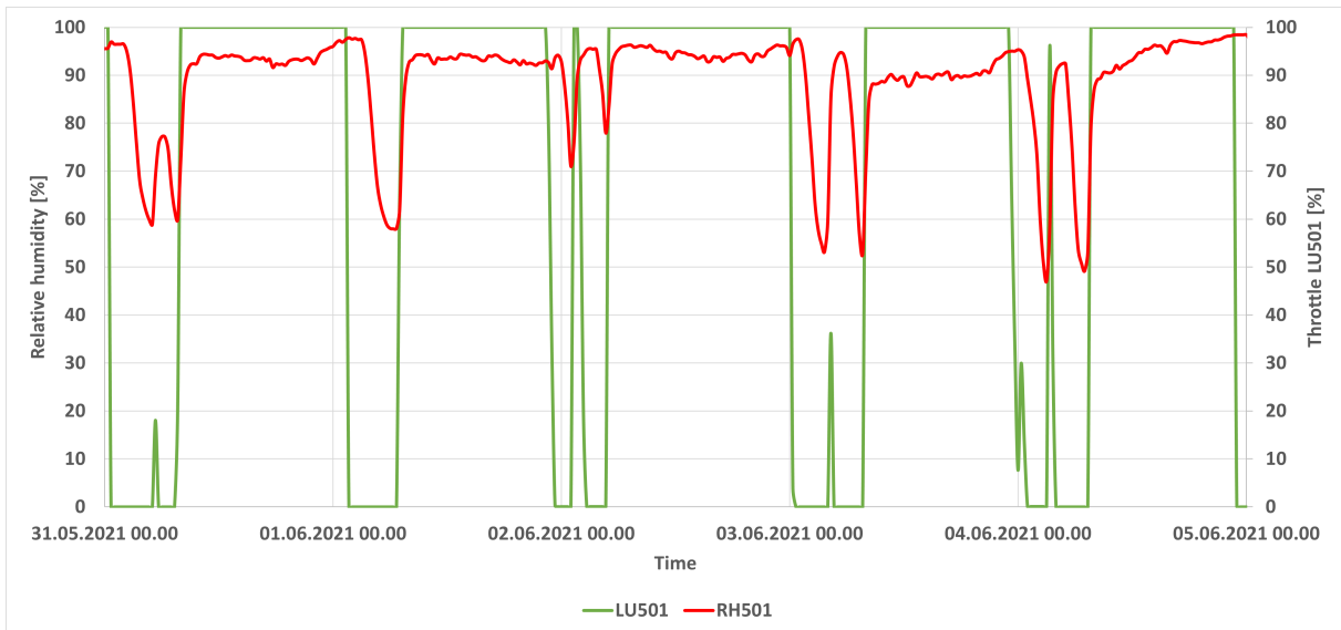
Figure 4.5: Throttle of humidifier LU501 and relative humidity of air after humidifier.
