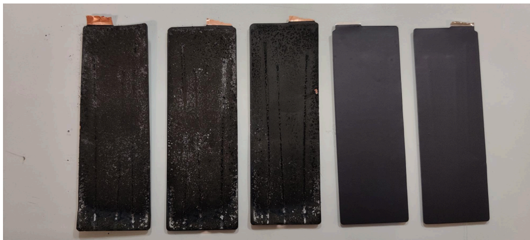
Figure 71: Image of anodes to the left and cathodes to the right, from an aged cell.
