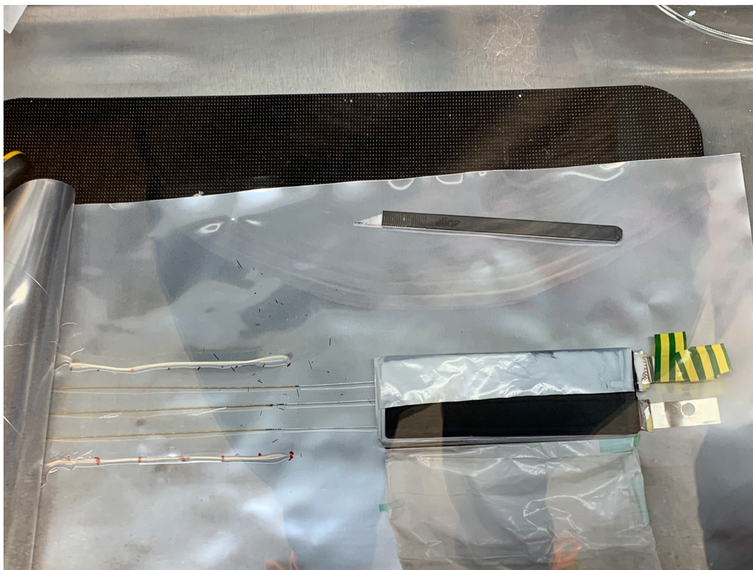
Figure 27: Image showing the insertion of the glass capillaries into the middle of the pouch cell battery. After insertion, the battery was slid to the left between the marked boundaries.
