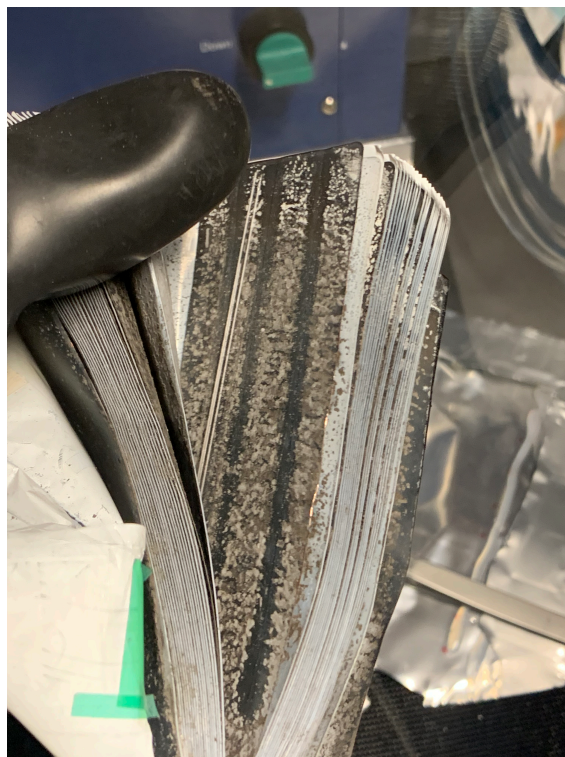
Figure 69: Traces of the glass capillaries on the anode surface where the glass capillaries were placed.
