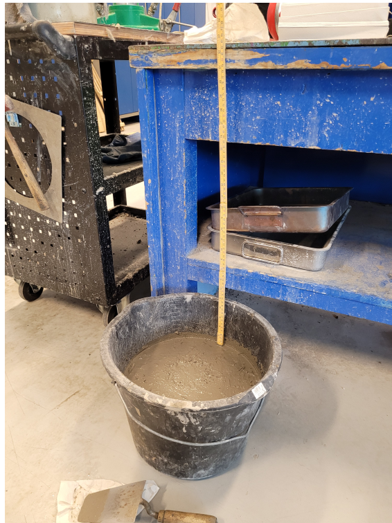
Figure 3.11: Picture of 20 L bucket with fresh concrete the prototype was dropped into during testing.
