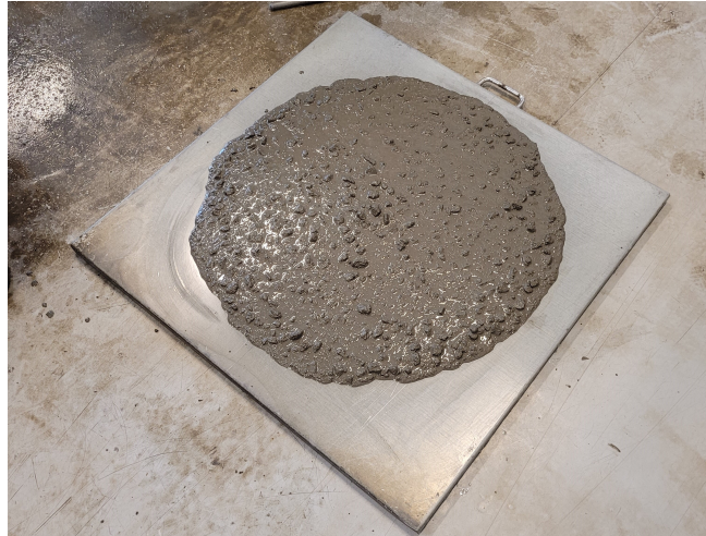
Figure 2.2: Slump flow test concrete spread.
