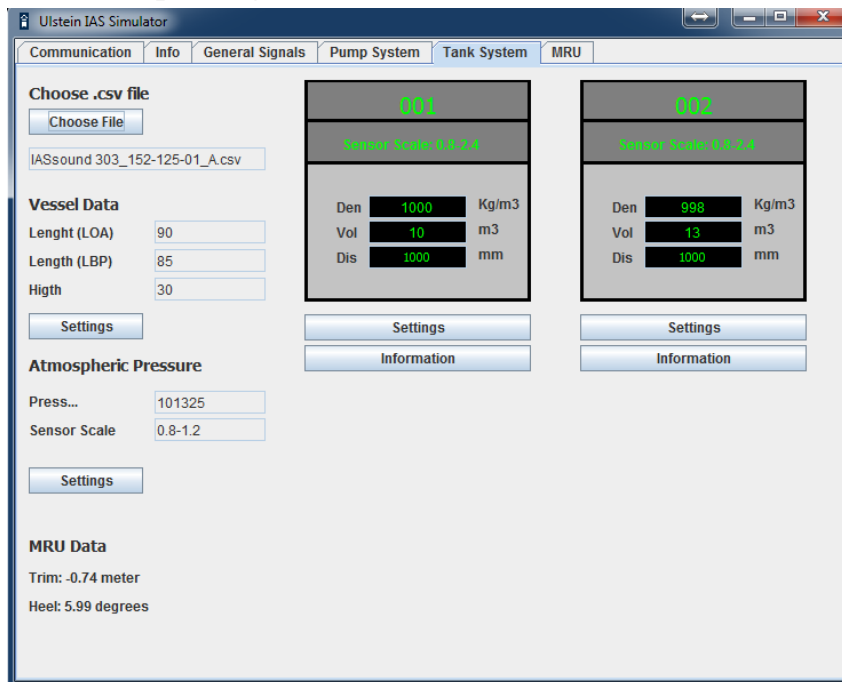
Figur 31: GUI tank system
