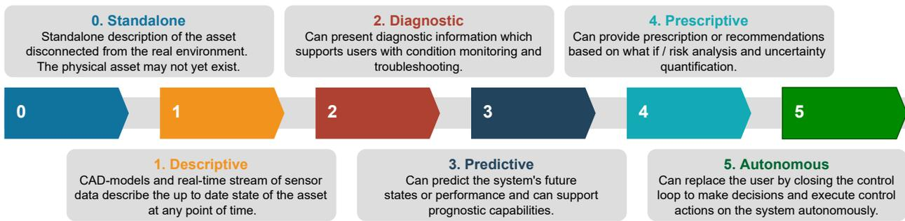
**Figure 2.2:** The capability levels of DTs on a scale from 0 to 5
