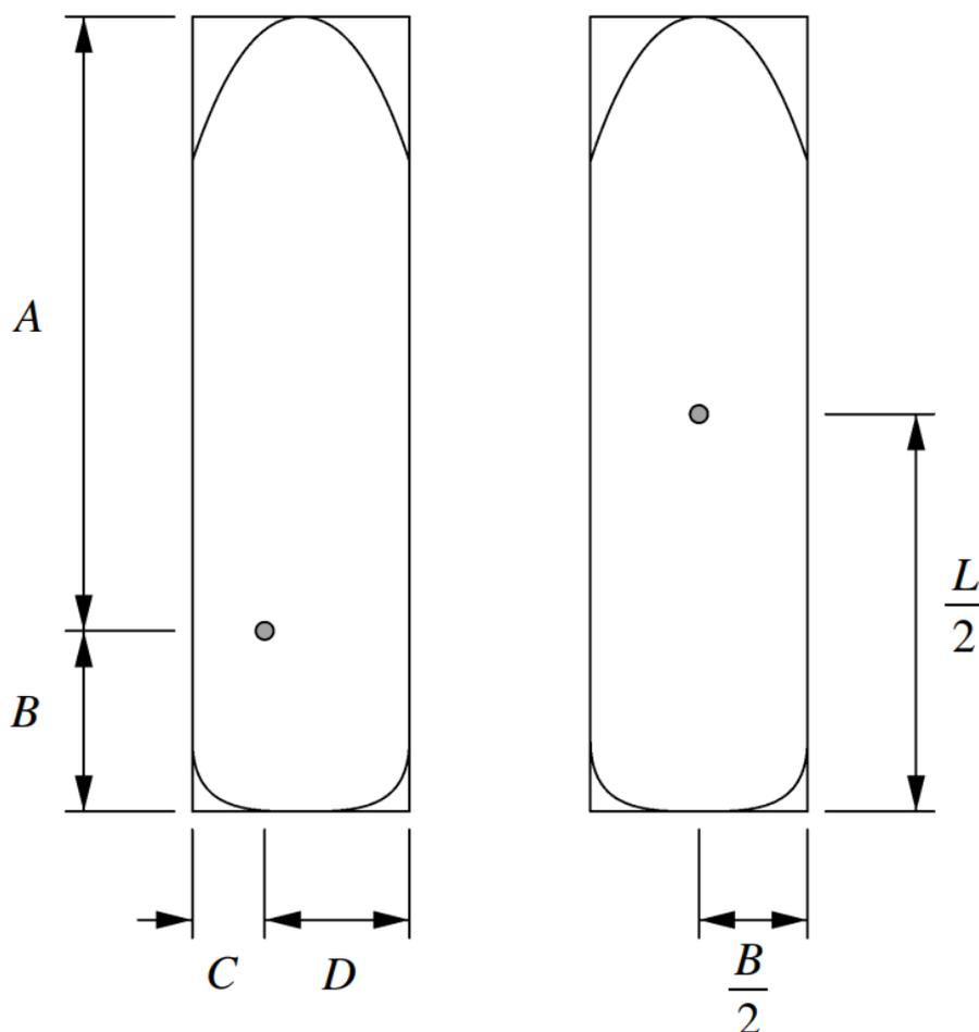
**Figure 2.8:** The dimensions A,B,C,D provided by the AIS. Courtesy of [18]
