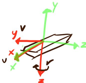
**Figure 2.4:** The coordinate system for the dynamical model (red) and Unity's coordinate system (green)
