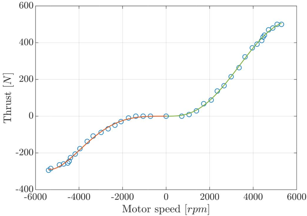
**Figure 2.6:** Thrust relative to RPM. Courtesy of [4]
