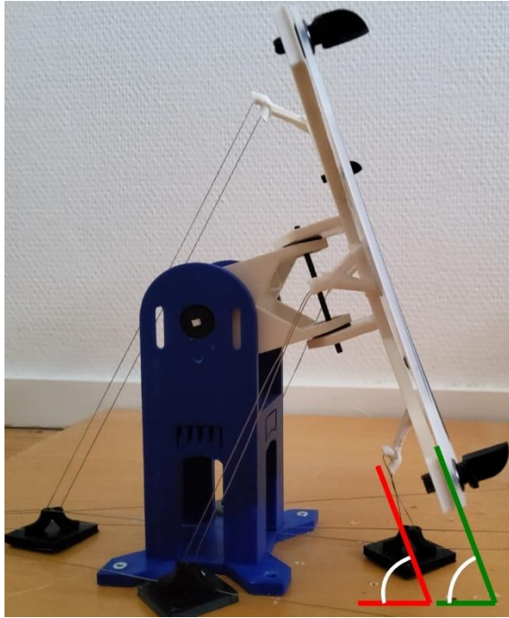
Figure 32: Limit state at maximum torsional moment
