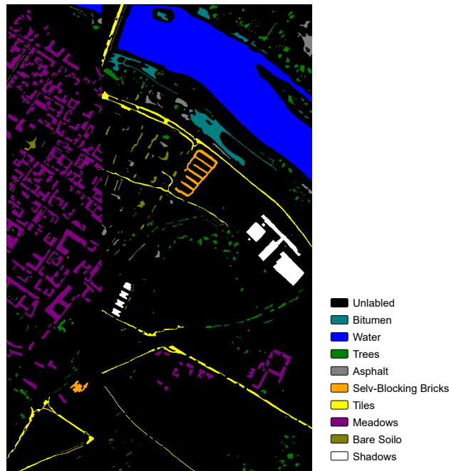
Fig. 3.7: Image showing the labeled pixels for the Pavia Centre scene presented in Figure 3.6. Each class has its own color as described in the right hand class list.
