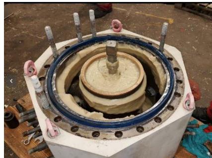
Figure 23 Open and inspection of Pig Diverter. Oil/wax slurry sample from different internal voids was collected to look for sand deposits
