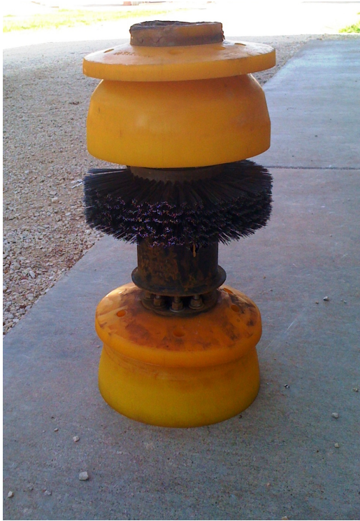
Fig. 1.1—A six-inch pig. ICberg7, CC BY 3.0 US < https://creativecommons.org/licenses/by/3.0/us/deed.en >, via Wikimedia Commons
