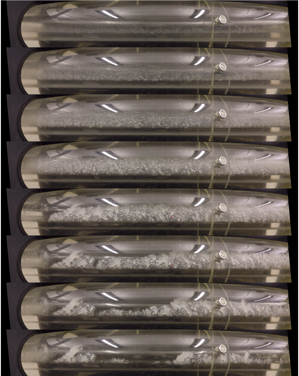
Fig. 4.18—Deposit evolution in stratified flow conditions.
