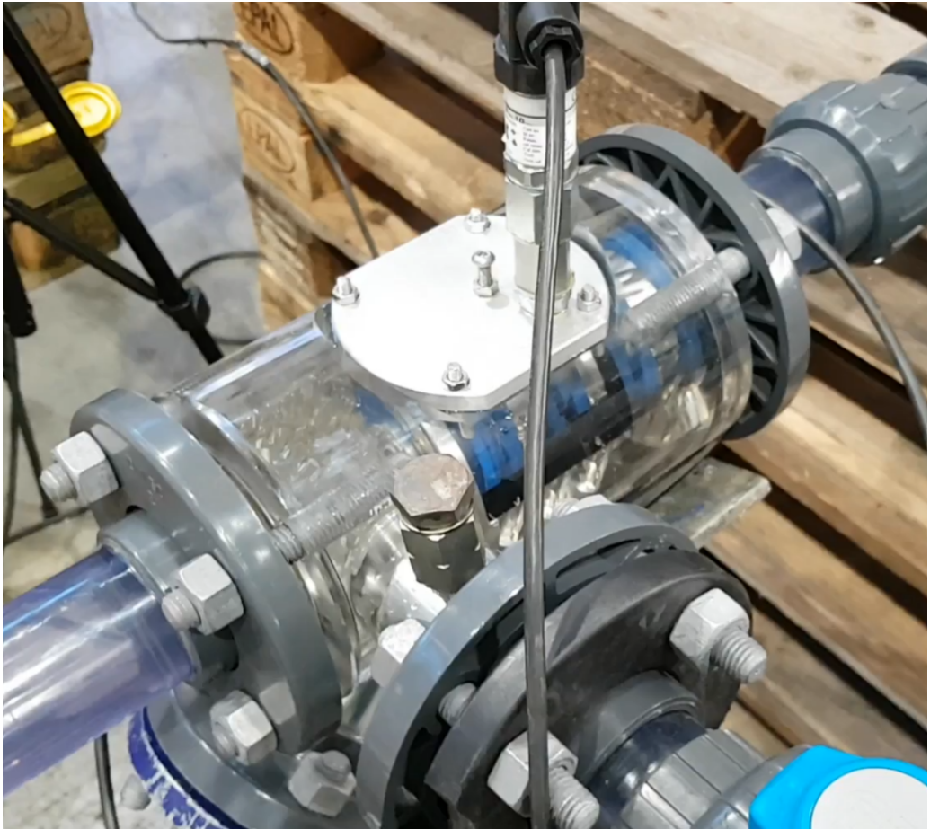
Fig. 2.6—Pig (blue item) stuck in the modified valve.
