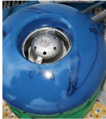
Figure 12 Front of Cleaning Pig with scratches and imprints (marked with black marker) from collision with partly opened valves.
