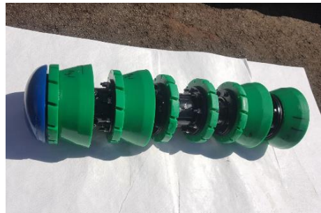
Figure 10 Cleaning Pig. Articulated 3 section design.
