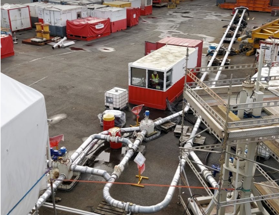
Figure 8 Wax Control System Qualification Rig. Approx. 120 m 6" pipe. Picture show AMPL (right side), Pig loop, Pig Diverter, control container, Pig Station and Flow Directional Valve.
