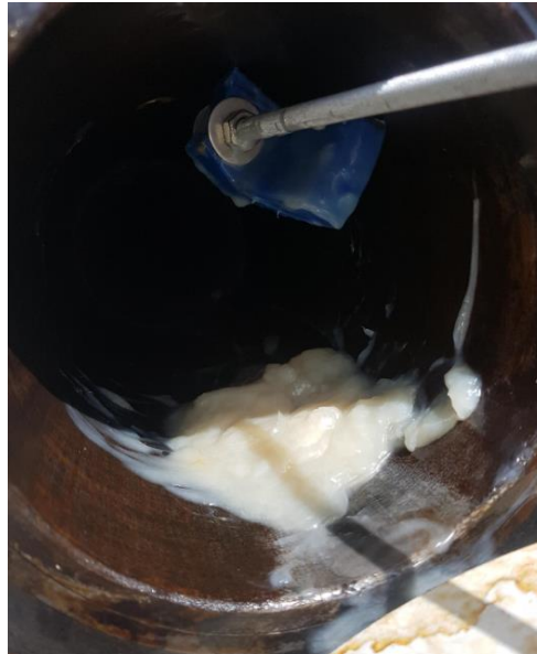
Figure 27 Amount of wax after normal wax production. Weight=165g
