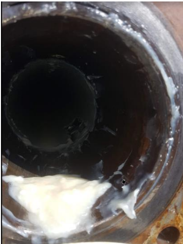
Figure 16 Wax layer after 3-hour cooling from 55°C to 15°C in rig. Wax was scraped from reference area inside pipe and weighed.
