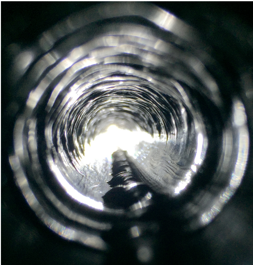
Fig. 4.15—Deposition in stratified flow case 2a.
