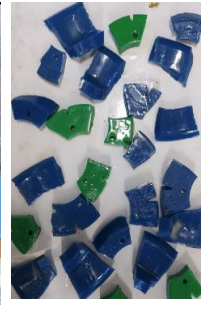
Figure 15 Parts of broken seal ring and guide ring that was sent in the flow through the Pig Diverter.
