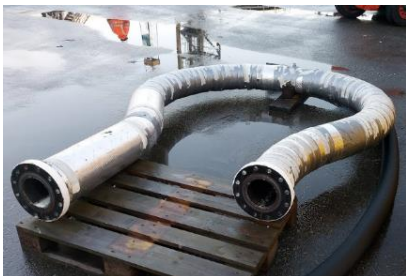
Figure 24 Part of Pig Loop with 5D bends
