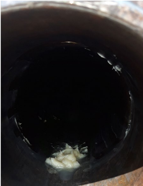
Figure 26 Amount of wax after cold flow test. Weight=11g
