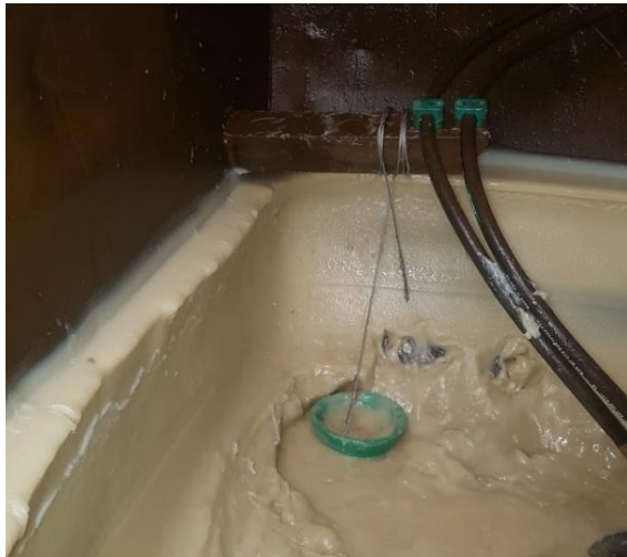
Figure 17 Oil/wax slurry in tank after cold night. Notice gel consistency. Also notice Cleaning Pig seal ring (green) that was stored in tank during test period
