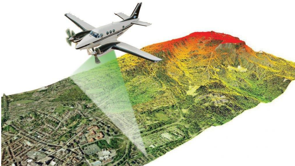
Figure 5: Airborne LiDAR -scanner that scans the terrain below (Laser kartlegging (LiDAR), 2021).
