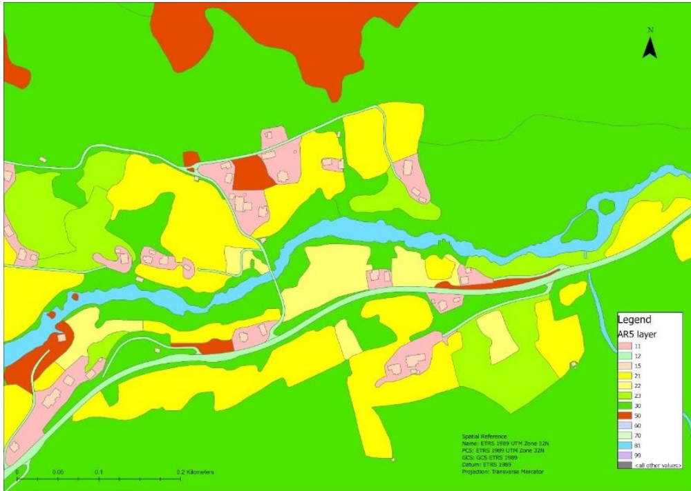
Figure 10: AR5 layer, with the Nibio codes given a separate color, and is connected to a Manning's N roughness value.
