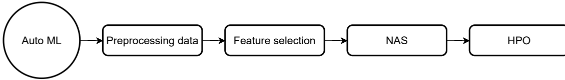
Figure 3.11: HPO in the AutoML chain. HPO aims to extract the maximum out of a model that already exists.
