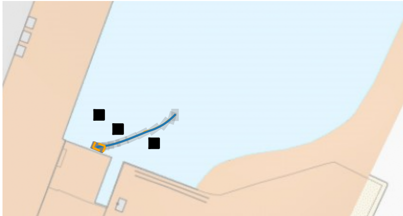
Figure 4.2.5: Method B's planned and executed trajectory from the initial pose to the dock pose for the closed-loop control scenario
