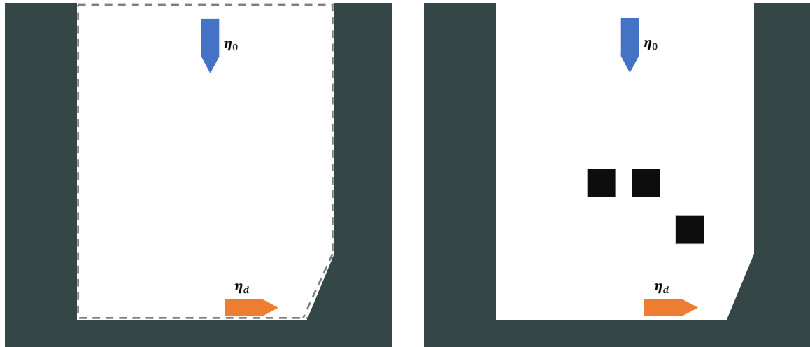
(1a) Initial problem where a convex polygon encloses the initial pose \eta_0 and the dock pose \eta_d
