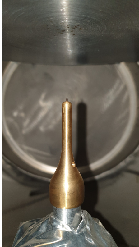
Figure 3.6: The rod-plane gap inside the tank. This configuration is 53 mm gap with needle.
