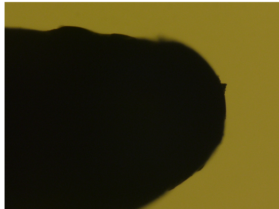
(b) The needle after many breakdowns during the specialization course.
