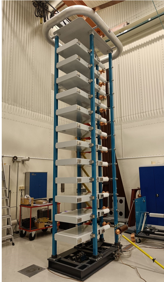
Figure 3.2: The 12 stage marx impulse generator
