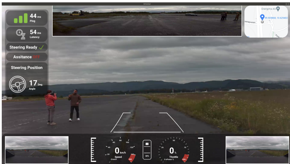
Figure 5.3: Operator's point of view in the GUI of the remote control system. Side cameras is changed to front wide cameras.
