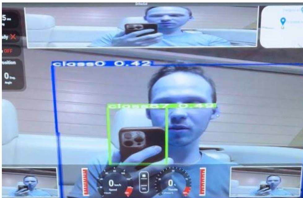
Figure 5.13: Testing of the implemented object detection with Yolo5, that is embedded into the remote control system as seen on picture.
