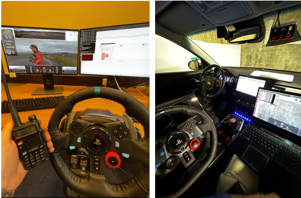
(a) Setup during test of the system in the office nearby the test track. (b) Setup inside the car during development and tests.
