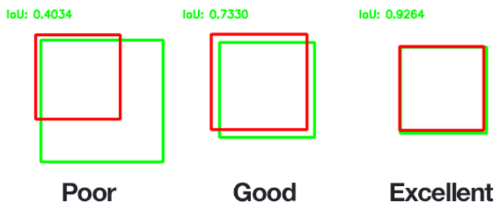
Figure 2.6: IoU scores of object detection. The better the prediction, the higher is the IoU. (Source: [Adrian Rosebrock, 2017])
