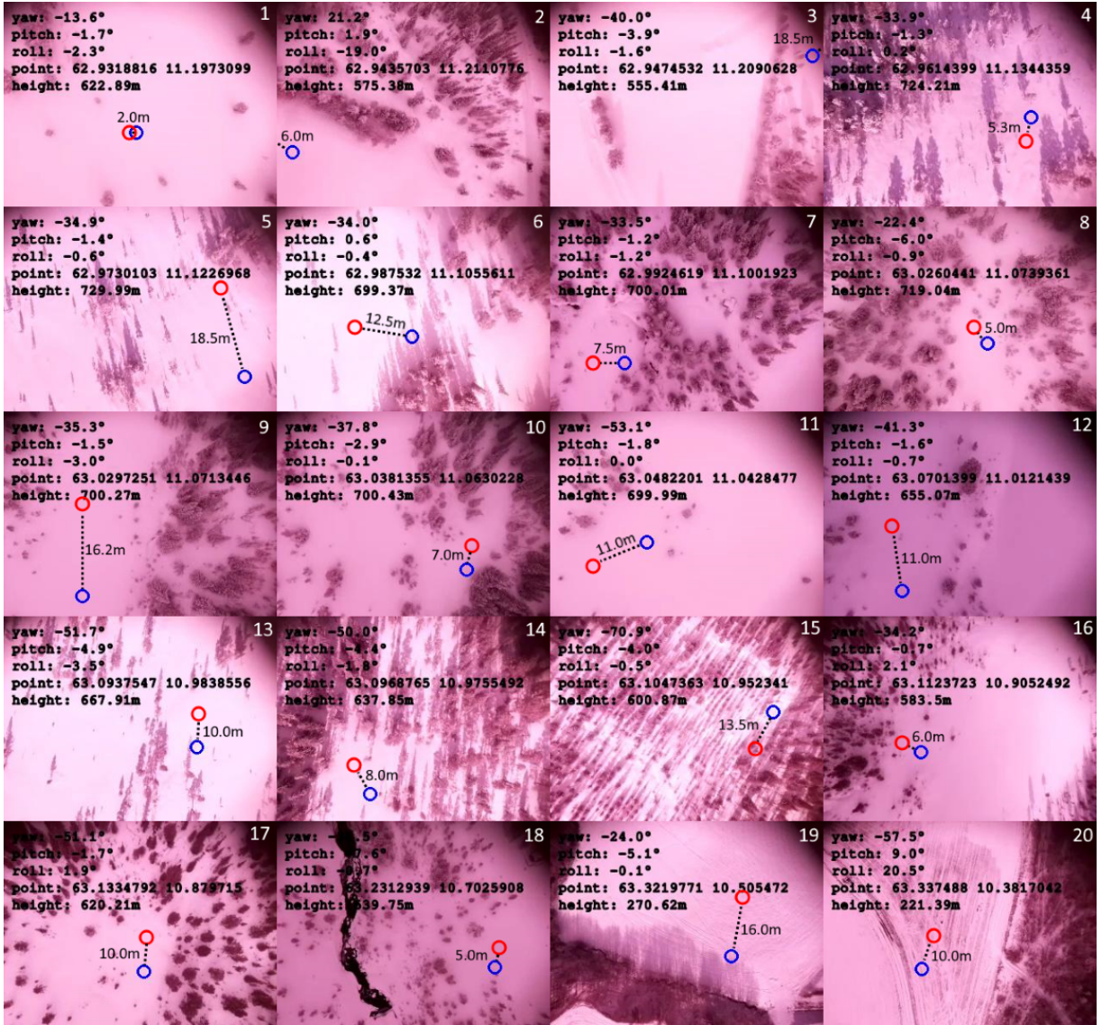
Figure 4.3: An overview of the accuracy measuring of the pixel geolocator. The point coordinate written in each image is the location the system claims the blue point is in. The red point is the actual location of the coordinate. The points are listed in Table 4.1.
