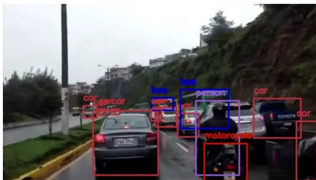
Figure 2.5: Example of object detection application: detecting cars on roads. (Source: [Hackem, 2020])
