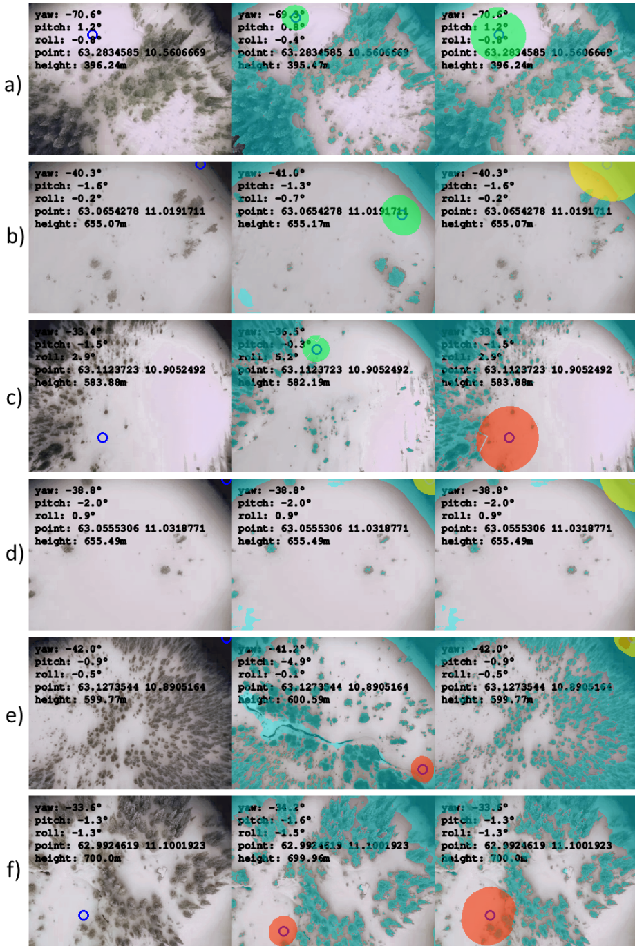
Figure 4.5: An overview of predictions from the rally point verification system. The leftmost column shows the hand-picked rally points. The center column shows the points covered by a circle with a radius of 10m. The rightmost column has circles with a radius of 20m. The points are evaluated based on the area of the circle. If the circle is green, the rally point is considered to be safe. If it is red, it means the point is considered unsafe. Yellow means that the entire circle is never completely inside any images in the video, and can therefore not be evaluated.
