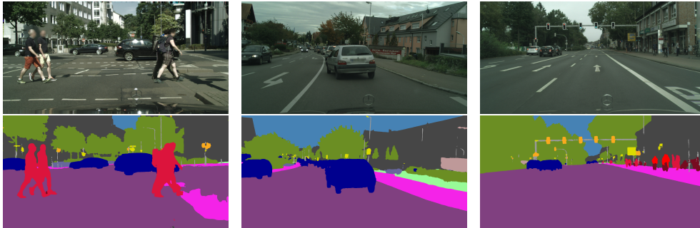
Figure 4.2: Experiment 0: Cityscapes qualitative results. First row: original image, second row: predicted segmentation mask.
