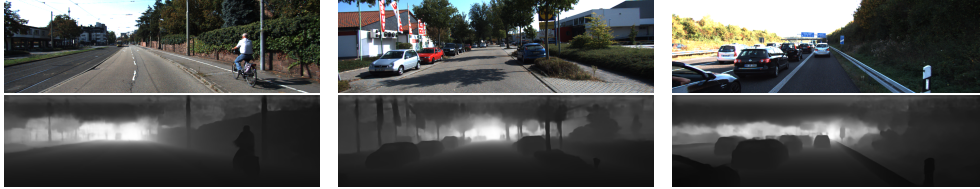
Figure 4.4: Experiment 0: KITTI qualitative results. First row: original image, second row: predicted depth map.
