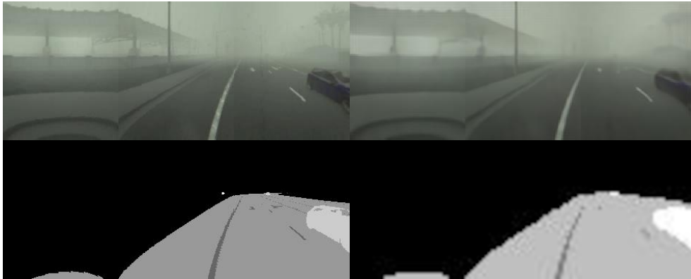
Figure 3.9: Figure showing input wide RGB, and its ground truth semantic segmentation on the left, and reconstructed wide RGB and predicted semantic segmentation image on the right. Images are taken from the validation step at epoch 12. The predicted semantic segmentation image is shown in its state prior to up-scaling using interpolation.
