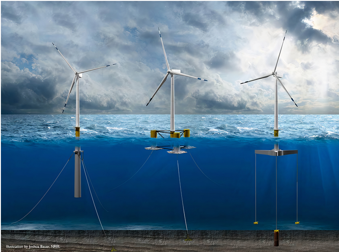
Figure 1.2: Different types of floating foundations, from left to right: spar, semi-submersible, TLP. Illustration by Joshua Bauer, National Renewable Energy Laboratory (Joshua Bauser, 2020).
