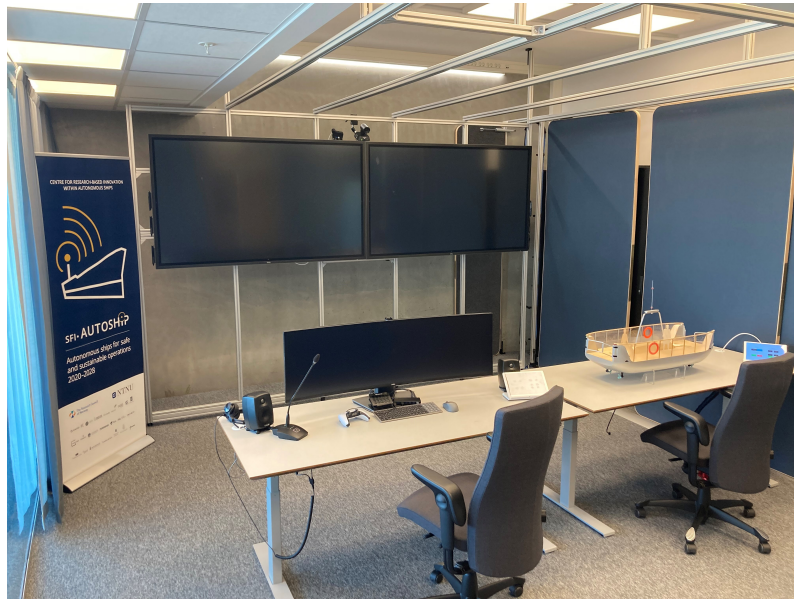
Figure 4: The Shore Control Lab located in Trondheim Maritime Center. The aluminum profile structure is meant to allow for rapid prototyping of different control room configurations. Source: Robin Stokke
