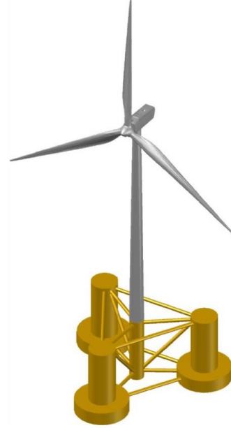
(b) OC4-DeepCwind applies a steel foundation [16]
