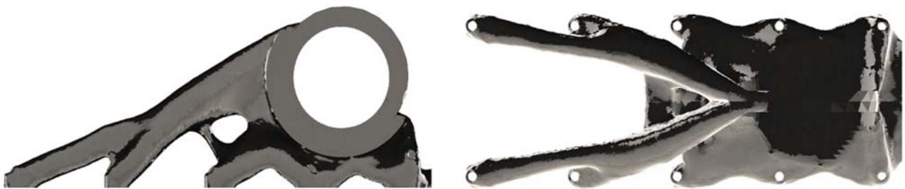
Figure 11: Final geometry of the case-study part after smoothing operation.
