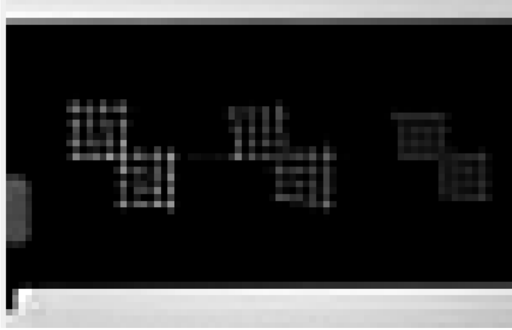
Figure 3.6: Image of the the arrays of holes in slice one used to assess the high contrast spatial resolution.
