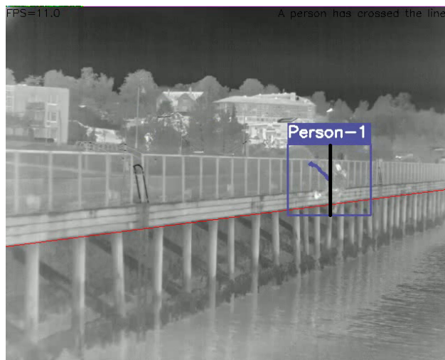
Figure 4.10: Line crossing check
