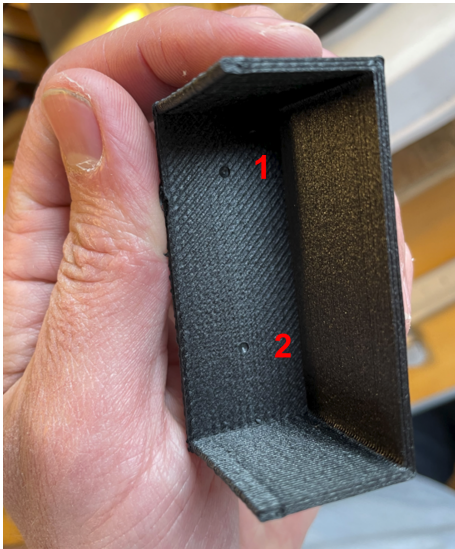
(a) Melt test specimen with drilled pits. Numbers showing placement of thermocouples 1 and 2.
