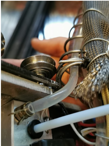
(a) Steel spring resting on the roller, causing friction.
