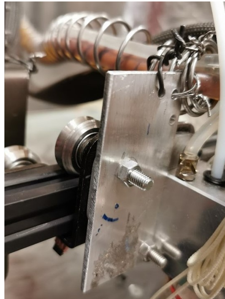
(b) Aluminium plate mounted to keep the steel spring away from the rollers.
