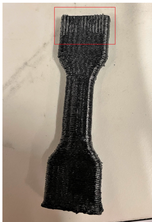
Figure D.4: Slip marks after cancelled tensile test.
