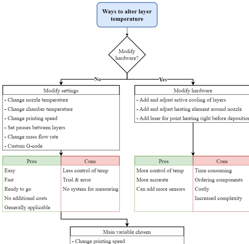
Figure 1: Diagram showing the two main approaches considered to alter layer temperature.
