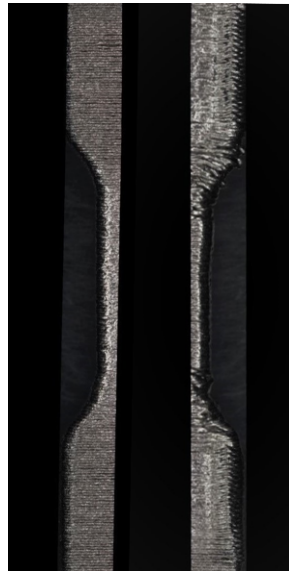
Figure B.2: Geometric differences, printer speed 7 mm/s (left) and 25 mm/s (right).
