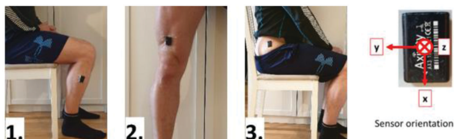
Figure 1. Sensor placement on: 1. lower leg, 2. thigh, and 3. hip, as well as the sensor orientation seen in all images. The arrows show the direction of positive acceleration with x pointing downward, y to the side, and z into the limb.
