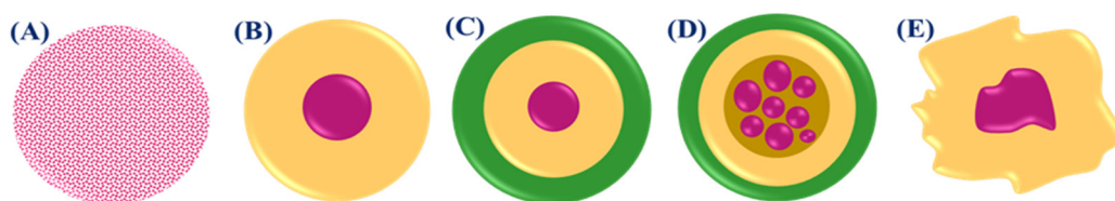
Figure 2. Schematic illustration of various morphologies formed by microencapsulation: microsphere (A), monolayer and mononuclear microcapsule (B), multilayer and mononuclear microcapsule (C), multilayer and multinuclear microcapsule (D), and microparticle (E).
