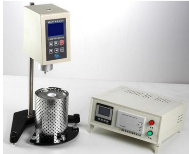
Figure 4. Brookfield rotational viscometer, which consists of two parts: a temperature control system and a shear rate control system.
