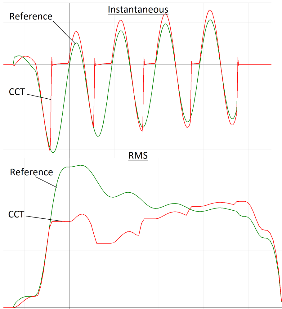
Figure 14: Core saturation of current transformer, Instantaneous values and RMS values.
