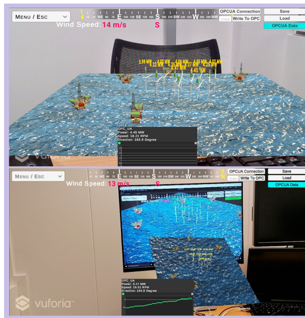
Figure 33: Augmented reality visualization view of digital twin of wind farm.
