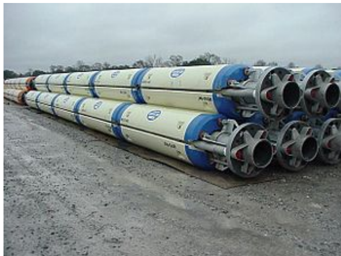
Figure 4: Picture of some riser joints with buoyancy modules [1]
