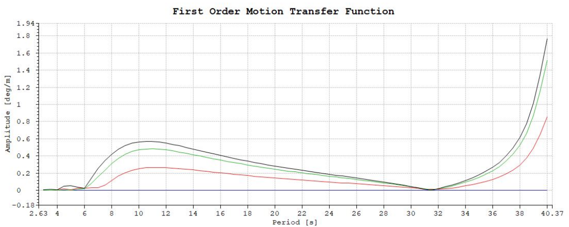
Figure 59: First order motion transfer functions for Ocean Vanguard. The blue curves corresponds to waves at 0 degrees, the red curves to 30 degrees, the green curves to 60 degrees and the black curves correspond to waves coming at 90 degrees angle
