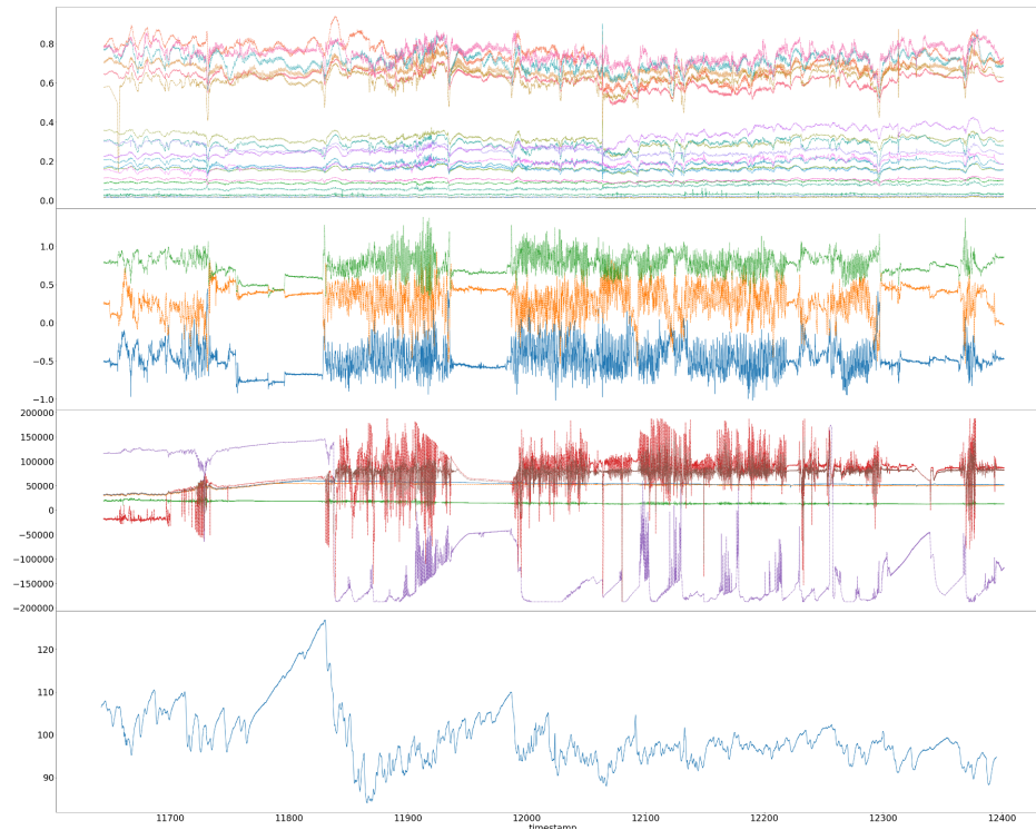
Figure 8.2: All sensors synchronized to the same timestamp, with fNIRS displayed at the top, then EEG_AUX, EEG, and lastly GSR
