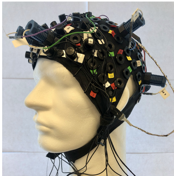
Figure 6.2: The cap with EEG electrodes and fNIRS optodes integrated
