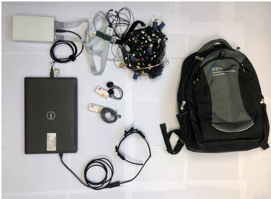
Figure 8.1: The complete experiment setup for the in situ experiment. The laptop and fNIRS device (white box) were placed in the backpack, the ECG in the participant’s front pocket, and the GSR in their hand.
