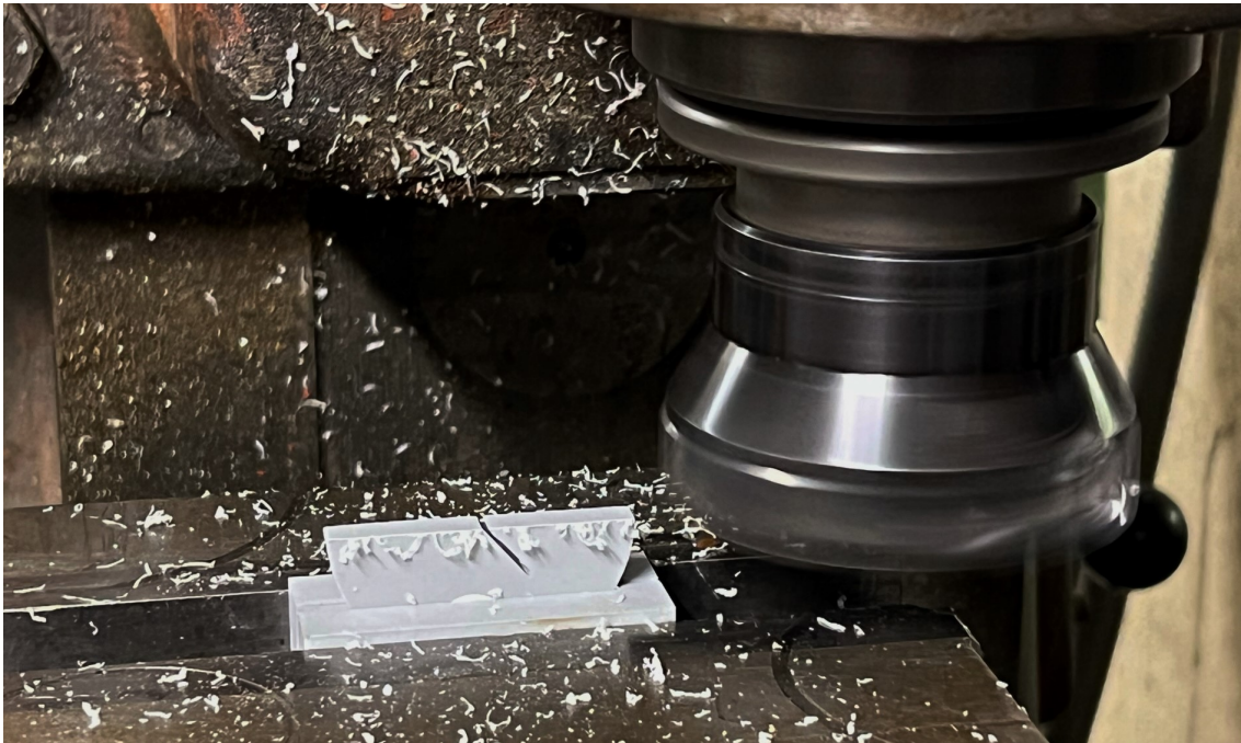
Figure 23: SCB-specimen mounted in mill and machined.
