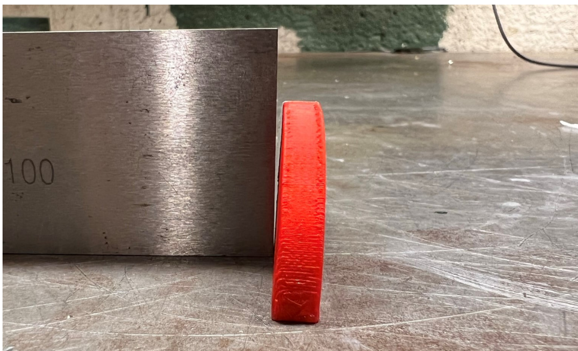
Figure 16: SCB-specimen with slanted cut after laser-cutting.
