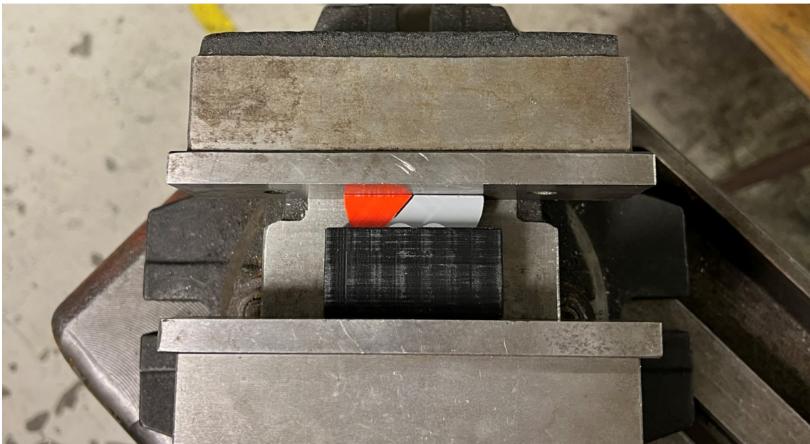
Figure 22: SCB-specimen loaded in fixture with vice.
