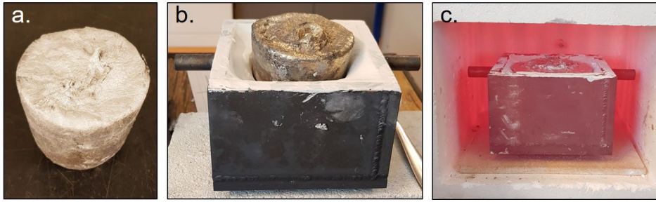
Figure 3.5: Photographs showing critical parts of the compression testing setup of filter samples submerged in molten aluminium: (a) a solidified metal sample with a primed filter sample submerged within, (b) a metal sample placed in the prepared container, and (c) melting of the metal sample in a resistance furnace before compression testing.
