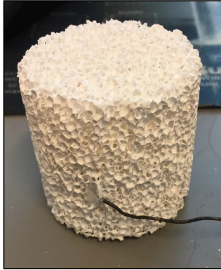
Figure 3.4: An example of how the dummy samples were prepared by inserting a thermocouple to record the temperature development within the filter samples.
